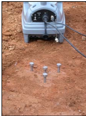
Fig. 17: Field probe rods after removing the template.
