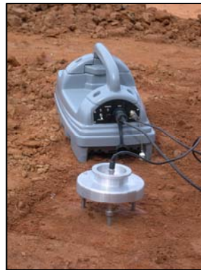
Fig. 18: The MRP Head is placed on top of the probes.
