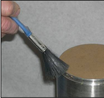
Figure 7 – Ensure the electric contact surfaces are clean.
