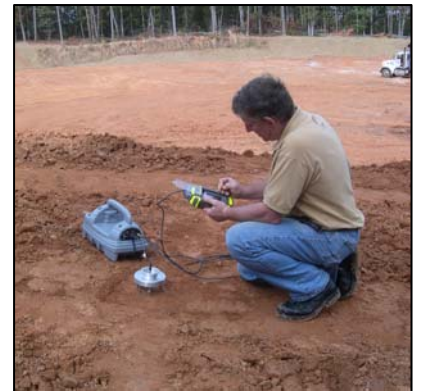
Fig. 19: Take a TDR measurement.
