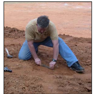
Fig. 13: Smooth the soil surface
