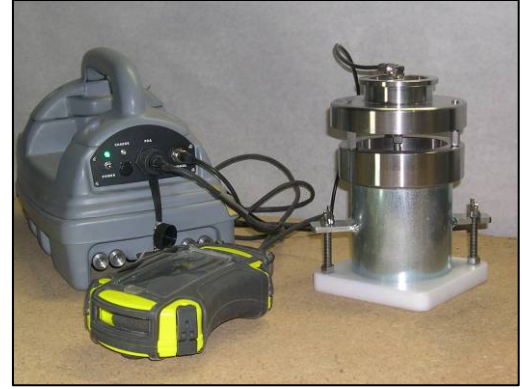
Figure 6– Take TDR reading.
