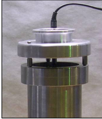
Figure 5 – Place the mold collar on the mold. Sit the Coaxial Head on the mold collar. Ensure the contact surfaces are clean (see Fig 7)
