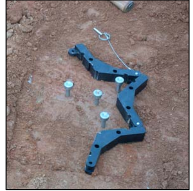
Fig 16: Remove the template by prying it open. Probes are exposed.
