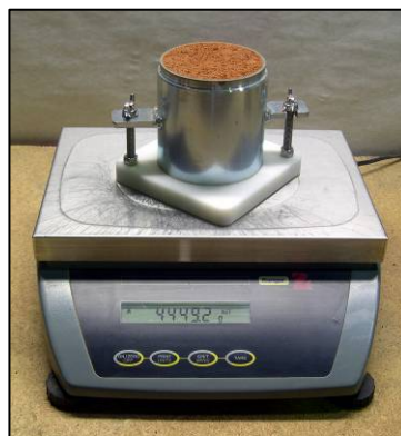
Fig. 2: Weight the soil specimen and mold to nearest gram (ASTM D 689).
