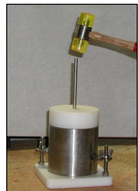
Fig. 3: Drive the center rod.
