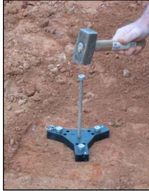
Fig 15: Drive the field center rod last.
