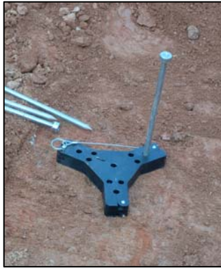
Fig 14: Drive the outer field probe rods first.
