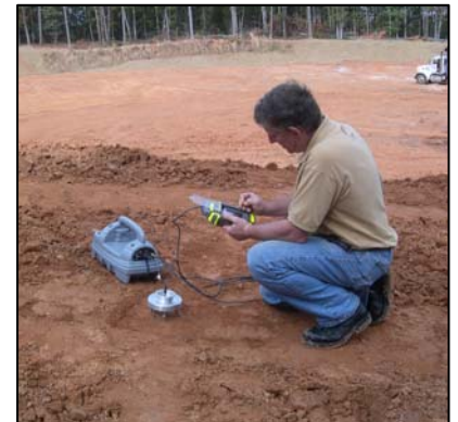
Fig. 19: Take a TDR measurement.
