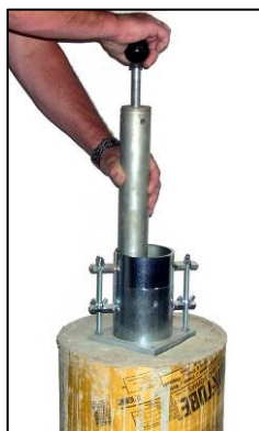
Fig. 1: Compact the soil (ASTM D 698).
