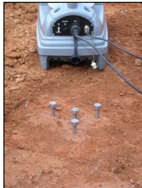
Fig. 17: Field probe rods after removing the template.
