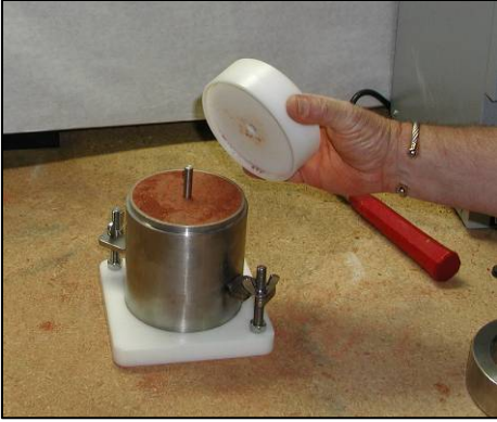
Figure 4 – Remove the guide for center rod and leave the center rod in place.
