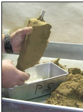
Fig. 9: Removing at least 0.5 kg (1lb).
