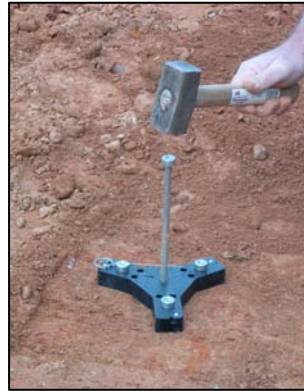
Fig 15: Drive the field center rod last.
