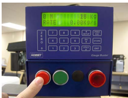
Press red start button to “jog” down
