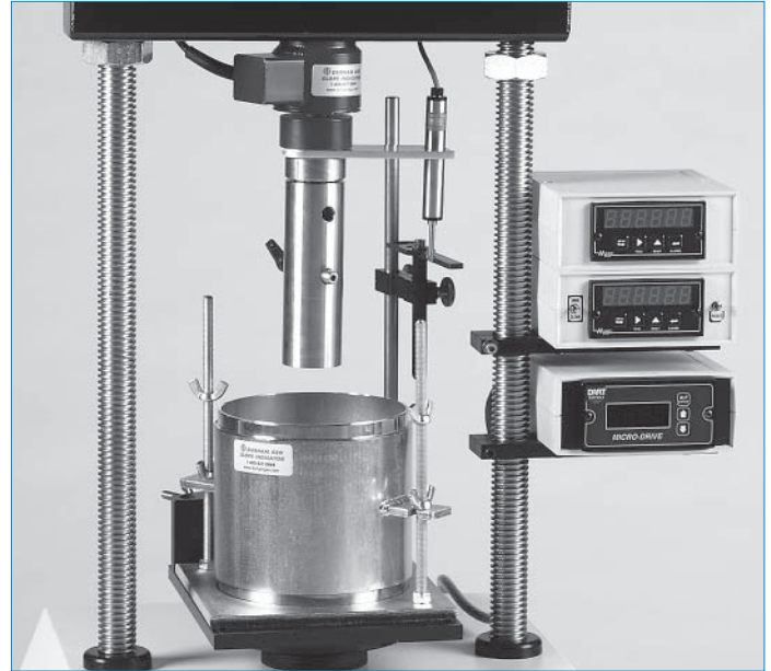
Detail of S-611 Auto Load Frame with accessories for CBR testing. Same accessories as on the illustration below plus the compaction mold, S-327.
