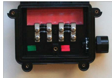
Electrical junction box, back of solar panel.
