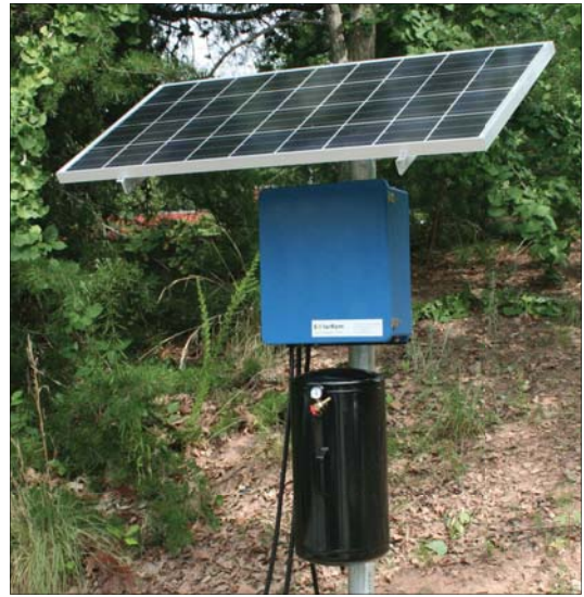
Front view of air tank mounted to pipe.
