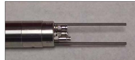
4. Place the rod skimmer on a flat surface and simultaneously pull all four tubes approximately four inches past the end of the connector tube (Note: the green tube is 4 inches long). When inserting the tubes into their fittings, do not twist the tubes over each other.
