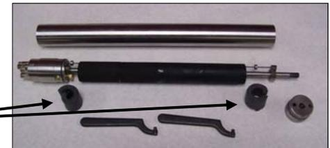
3. Reassemble the pump then unpack the P.O.D skimmer. Remove the washers and acorn nut from the threaded rods located at the bottom of the skimmer and thread them into the pump as shown. Insert the threaded rods into the head 1/4 inch.
