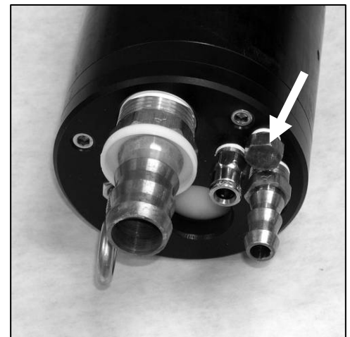
The arrow indicates the plug head to be removed
