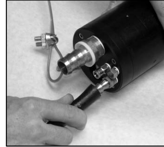
Connecting the air exhaust line
