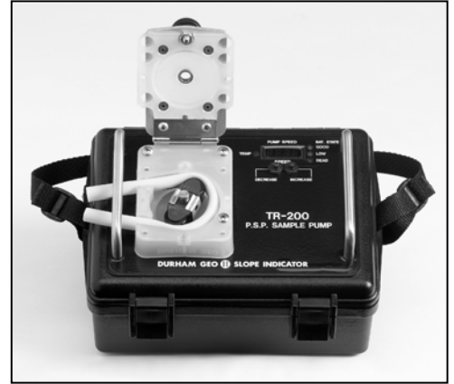
Fig. 1: To replace the pump tubing, flip the pump cover open to gain access to the roller.
