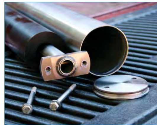
Top-loading pump, TR-974, disassembled.
